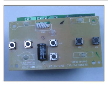
Lift the circuit board straight up to remove it from the base.
