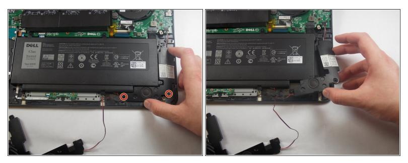
Start removing the right speaker by pushing the speaker in the direction of the tick marks on the 2
