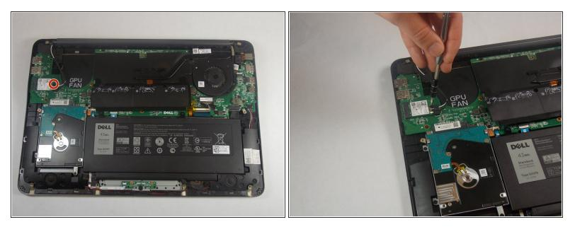
Remove the 3.0 mm-long Philips #0 screw at the end of the Wifi-Card
