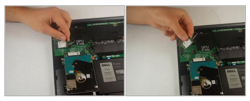
• Remove the Wifi-Card from its socket by pulling away and up from the connector.
