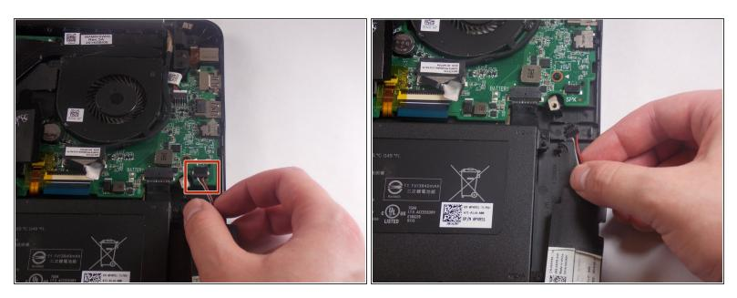
Remove the cable connecting the right speaker to the motherboard by pulling towards the front of the device.
