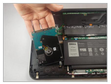
• Lift the hard drive out of the chassis.
