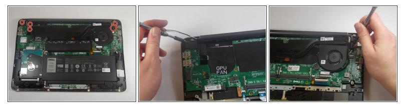
Remove the six 7.0 mm-long Philips #0 screws that mount the hinges.
