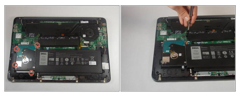
• Remove the four 5.0 mm-long Philips #0 screws connecting the hard drive to the chassis.
