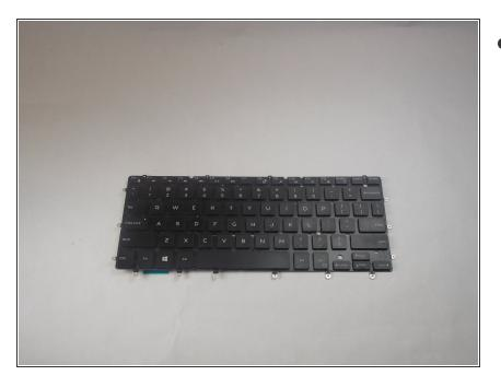
• Lift the the keyboard from the chassis.
