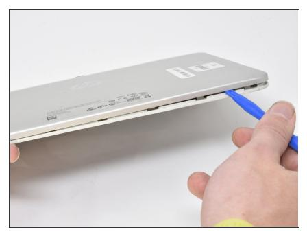
Slide the opening tool along the seam between the back panel and the screen panel, prying the panels apart as you move around the edges.
