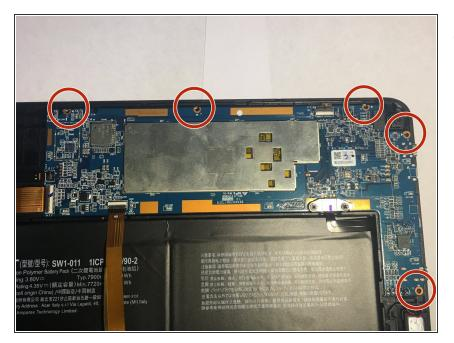
Remove the five screws on the outer edge of the motherboard using a Phillips #0 screwdriver.
