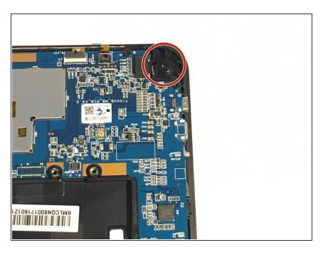
Locate the Rear Camera in the upper right hand corner of the motherboard.
