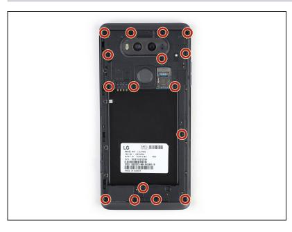
Phillips #00 screws attaching the back cover to the motherboard.
