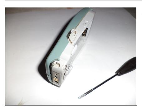
Remove the front cover with a small flathead screwdriver or case opener.
