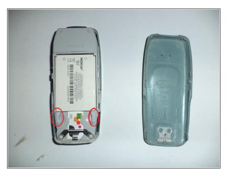
Remove battery cover, battery and SIM Card.
