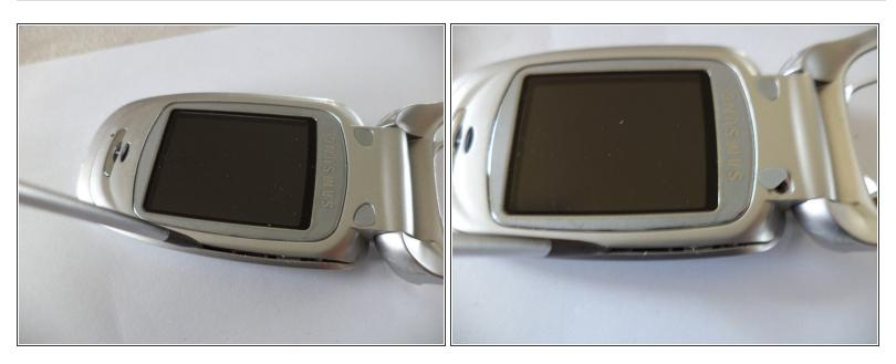
• To take the LCD display out of the case, click the upper case open with a small flathead screwdriver or case opener. Under the two pads under the LCD Display are 2 screws.
