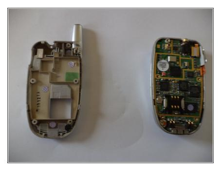
If the screws are removed, you can take the case of with your fingers or a small flathead screwdriver
