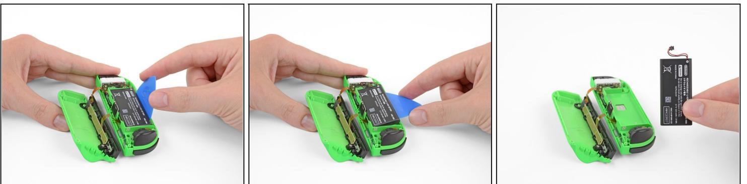
ⓘ The following two steps show the removal of the battery and the coaxial antenna cable from the midframe. **These two steps make for a less cluttered repair, but are not essential.** If you want, you can leave the battery and the grey coax cable in place here and proceed to [step 7](#).
