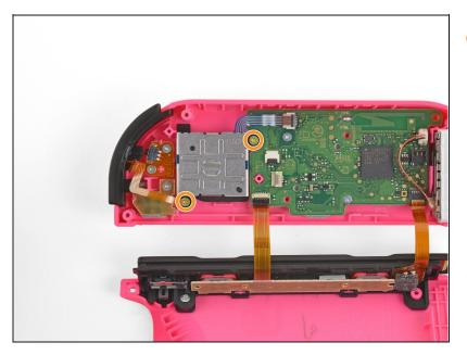
Remove the two 3.5 mm Phillips #00 screws from the joystick.
