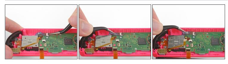
• Finally, the joystick is locked into place by one last ZIF connector. Carefully flip the ZIF lock upward and disconnect the cable.
