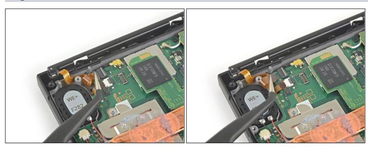
• Use a pair of <u>tweezers</u> to slide the Joy Con rail data cable out of its connector on the motherboard.
