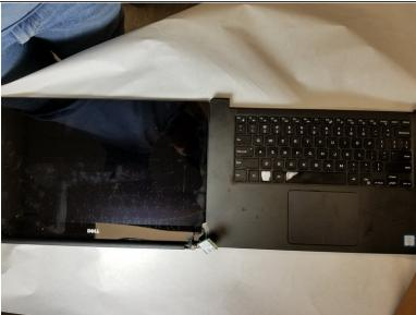
• Flip the laptop over, so it is sitting in the normal upright position. Hold onto the screen, and pull the keyboard up and away from the screen.
