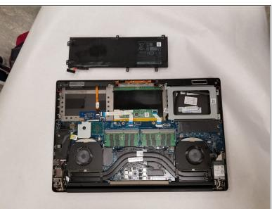
Carefully remove the battery from the computer.
