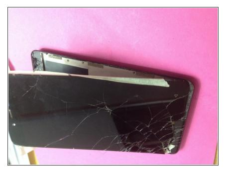
Using a heat gun or other tool to apply some heat to the screen, making the glue softing and using tool to separate the screen. Be carfully at the bottom where the flex connection.
