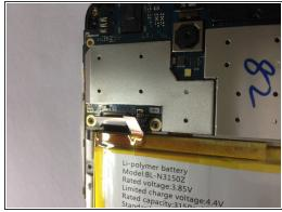
After removed the Back Plastic Cover, a metal bracket is covering the battery connector and the LCD screen connector. Removed all the screws in the metal bracket, then removed the Metal Bracket. Now, disconnect the two connectors of the LCD and Battery.
