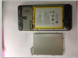
After the damaged LCD screen were removed, install the new LCD screen, remember the flex and connector need to go thought the small opening below the battery. Connecting back both connectors, and secure the metal bracket on top of the battery.
