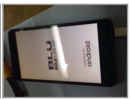
• After put back all the screws in the Metal bracket, time to test the new LCD Screen. Connecting the charger, to see the charging port is functional, then do a power on to verified the LCD Screen working or not. If both working as they should, job almost done. Now put back the Back Plastic Cover and we call it done.
