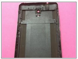
locate the edge the phone, to find a easy entre point, then using a Isesamo opening tool to open the four sides, and removed back cover.
