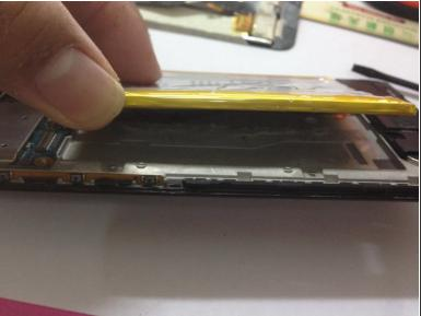
Here is tough part of all, the battery had two stripe of adhesive at tha bottom to secured it down. Just like the Iphone 6, you can carefully pull the adhesive stripe out or using tool to lift up the battery on the side where the connector of the battery located. After lift the battery up, disconnect the both connectors.
