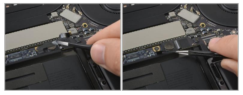
• Fold the battery board data cable to the side and out of the way.
