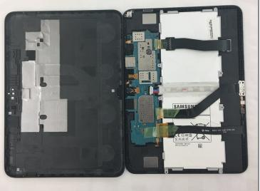
• Insert the wedge of the nylon spudger and slide it between the front and back panels until the back comes off.
