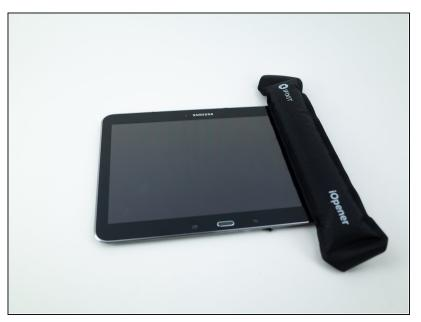
• Use an <u>iOpener</u> to weaken the adhesive around the display.
