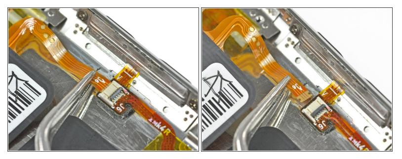
• Use a pair of tweezers to pull the control button ribbon cable straight out of its socket.
