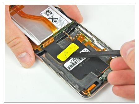
Use the flat end of a spudger to separate the Wi-Fi ribbon cable from the adhesive securing it to the rear panel.
