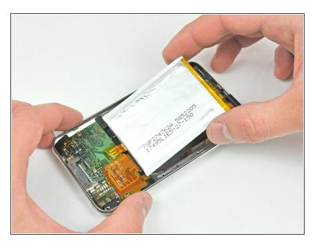
Gently pull the lower portion of the logic board away from the bottom edge of the rear panel.
