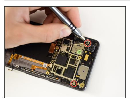
Remove the two 2.5 mm PH00 screws.
