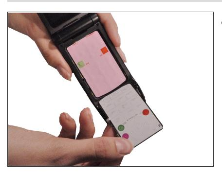
• Grasp the keypad membrane firmly and remove it from the phone.
