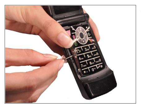
Continue working the pin under the keypad membrane until it is elevated enough to grasp.
