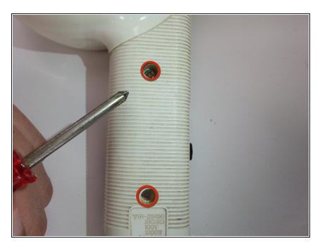
Using a Phillips #1 Screwdriver, remove the screws located on the hair dryer handle.
