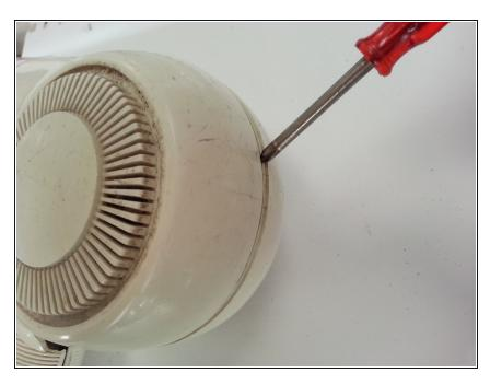
Using a <u>plastic opening tool</u>, carefully remove the front face of the hair dryer plastic case.
