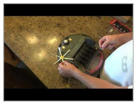
Just unscrew the side brush and put the new side brush in and screw it in.
