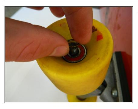
Slide the second washer onto the axle on the outside of the wheel.
