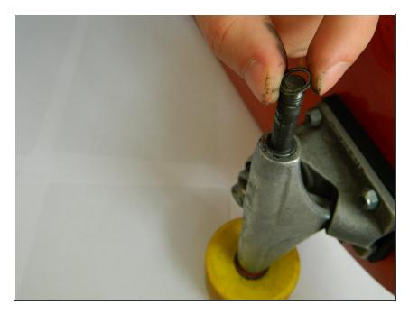
Slide one washer onto the axle.
