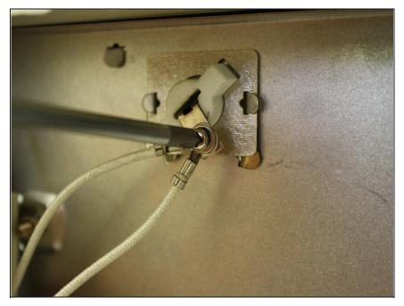
• Retighten screw to secure lead.
