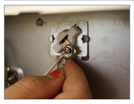
• Make sure that the lead is attached and in contact.
