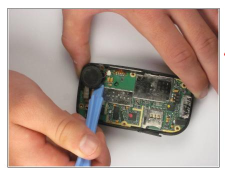
• Remove the speaker using a plastic opening tool.
