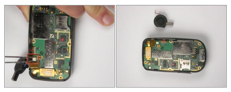
• Remove the wire attached to the speaker from the motherboard using tweezers.
