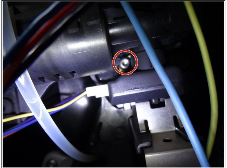
**i** The brew unit is mounted from the motor side with two Torx T20 screws to the left and right of the motor connection, these are located deep on the inside.
