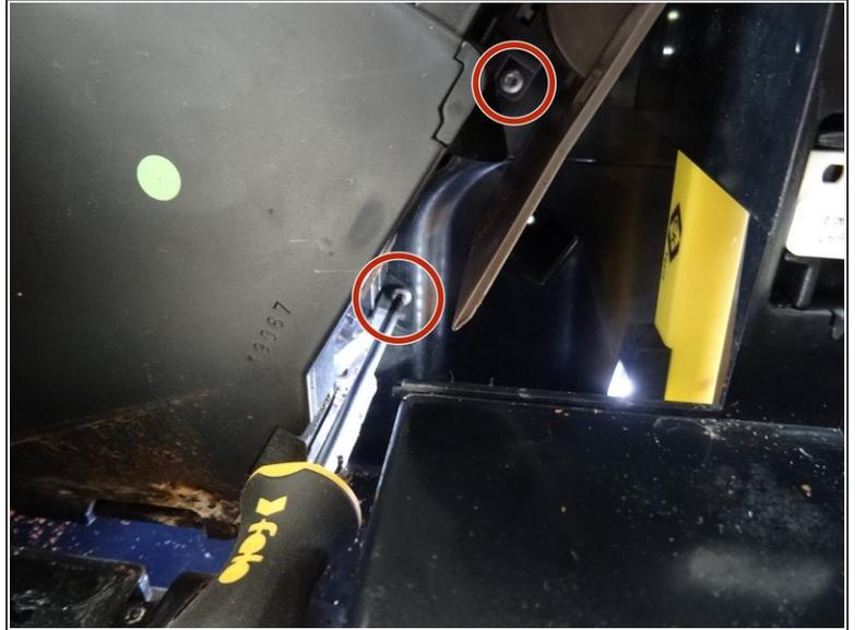
**i** The brew unit moves up and down in a slide driven by an elongated rack. There are four Torx T10 screws on the slide. The top left screw must remain attached.
