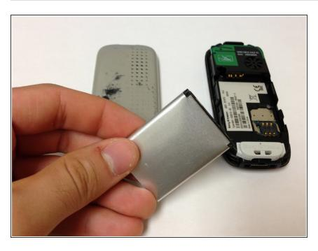
Remove the battery by wedging it out from the back.
