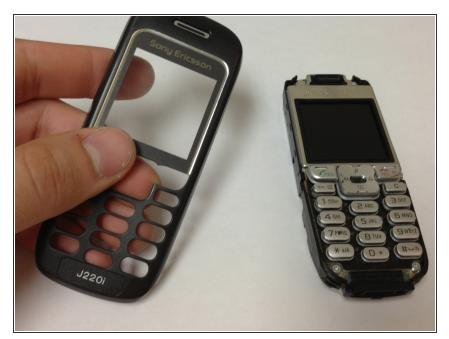
Flip to the front of the phone and apply pressure to the front frame of the phone. The frame should snap off easily.
