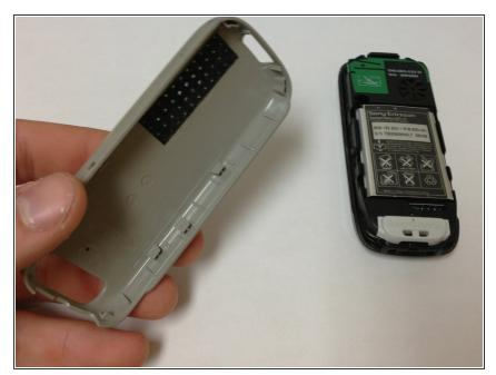
Firmly hold down the black button on the top of the phone and gently snap off the back cover.
