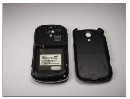
Pull at the plastic backing gently to remove it after hearing the snap sound.
