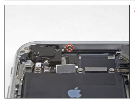
• Remove the 1.4 mm Phillips screw securing the antenna component to the top of edge of the case.
