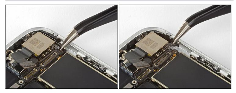
• Use <u>tweezers</u> to gently bend the logic board grounding bracket out of the way.
