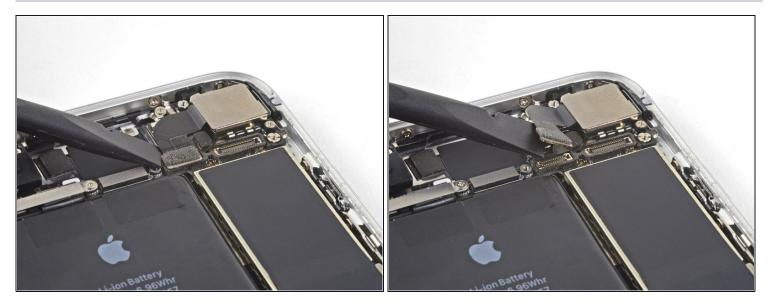
• Use the flat end of a spudger to disconnect the camera cable connector by prying it straight up from its socket.
