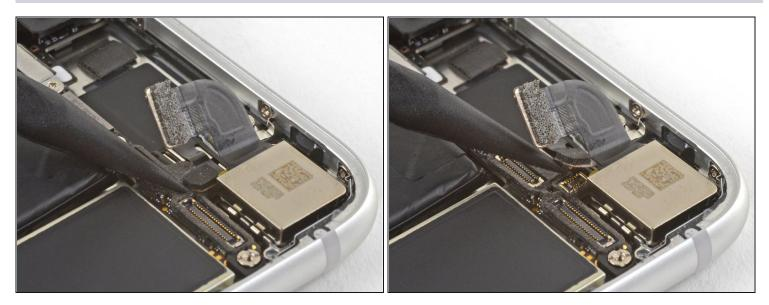
• Use the point of a spudger to disconnect the flash connector from its socket by prying it straight up.
