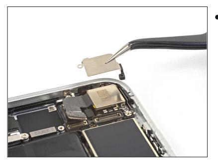
• Remove the rear-facing camera bracket.
