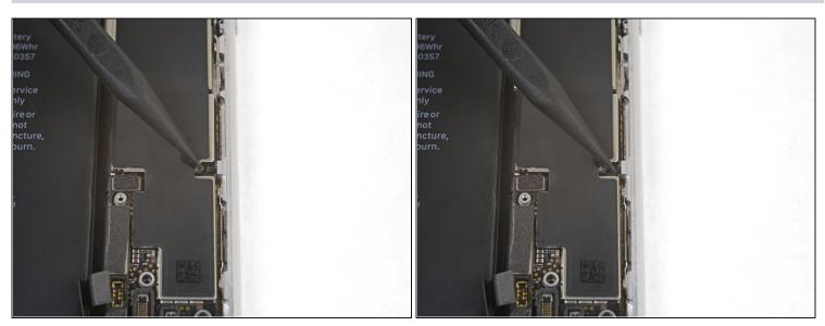
• Use the point of a spudger to move the SIM card eject plunger out of the logic board's way.
