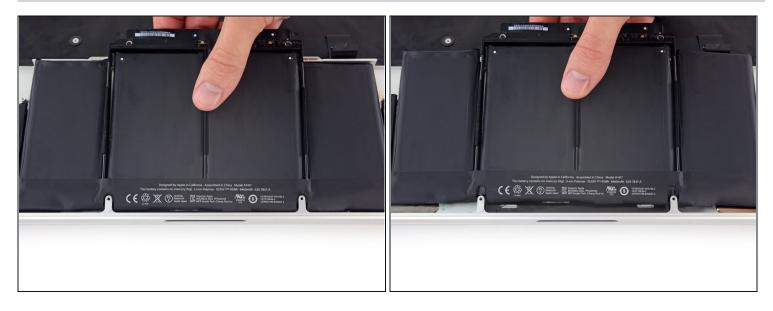
• Lift the battery with the plastic frame and slide it back toward the MacBook Pro's hinge until it clears the screw posts holding it to the upper case.
