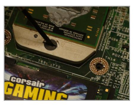
Remove the one Flathead #2.5 screw securing the CPU with a Flathead #2.5 screwdriver.
