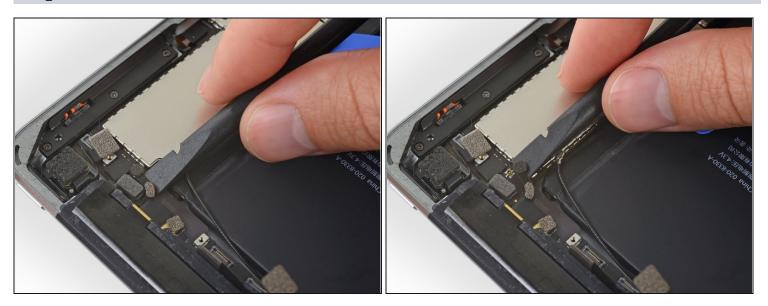
• Use the flat end of a spudger to disconnect the primary cellular antenna interconnect cable from its socket on the logic board.
