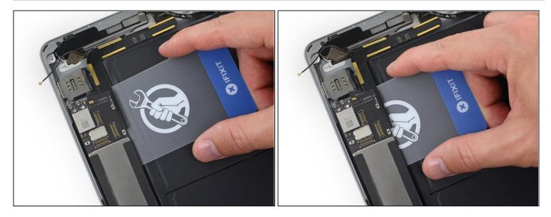
• Insert a plastic card underneath the lower end of the logic board, directly underneath the display connectors and Wi-Fi module.
