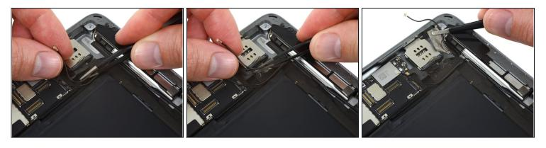
• Use a pair of tweezers to peel up the tape securing the right Wi-Fi antenna cable near the SIM board.
