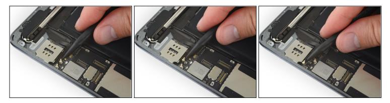
• Disconnect the left and right Wi-Fi antenna cables by lifting them straight up from their sockets on the lower end of the logic board.
