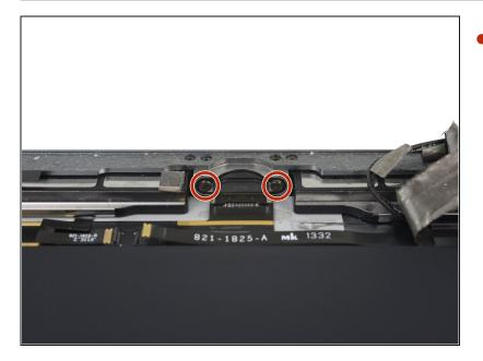
Remove the two 3.3 mm Phillips screws securing the Lightning connector to the rear case.
