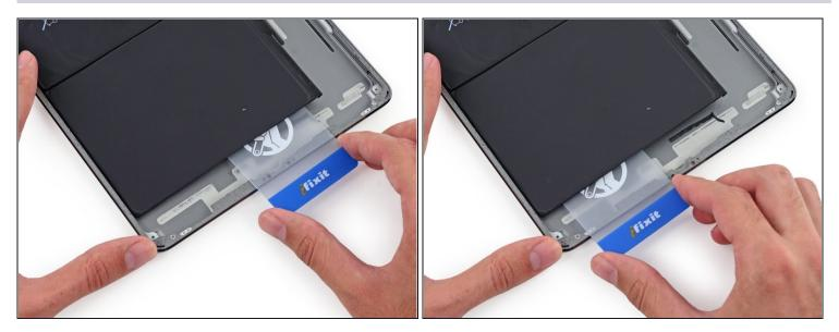
• Slide the plastic card to the lower left corner of the battery.
