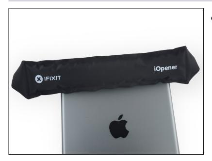
• Lay a warm iOpener over the upper edge of the iPad and let it sit for a couple minutes to soften the adhesive holding the logic board in place.
