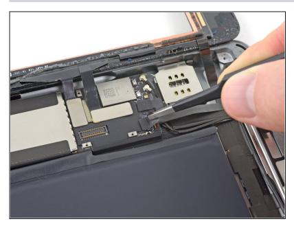
• Remove any tape covering the home button ribbon cable connector.
