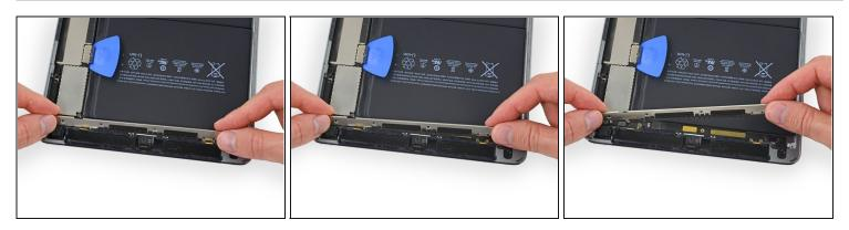
• Slowly peel the upper component cable bracket up out of the iPad—leaving the tape pieces on the bracket to make it easier to reinstall.
