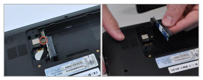
Underneath the computer, unscrew the hard drive connector screw, and pop out the hard drive plug-in.
