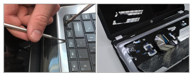
• Slide the tool that is now under the keyboard sideways along the edge and use another tool to depress the other tabs along the edge of the keyboard.
