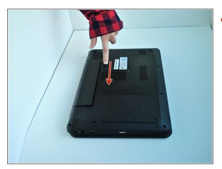
• Slide the switch under the battery compartment to release the battery.
