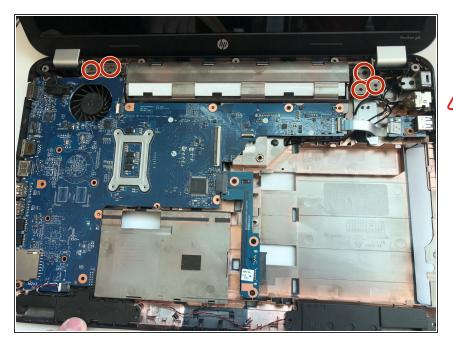
Remove the five screws holding hinges to base.
