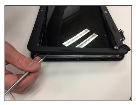
• Pry off the plastic surrounding the screen with any flat metal tool.
