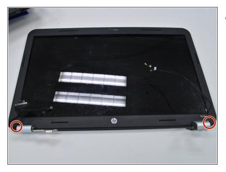
Remove the sticky tabs on the bottom of the screen just outside the hinges, and remove the two screws underneath.
