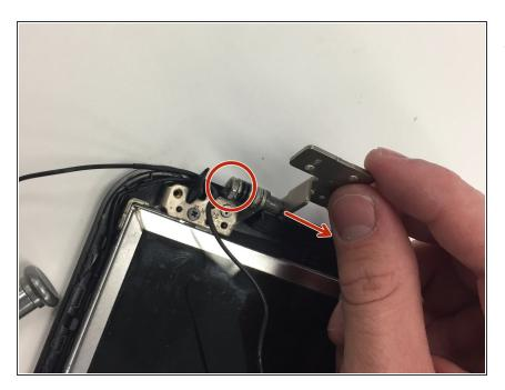
• Use a pair of pliers to unscrew the nut and pull out the hinge.
