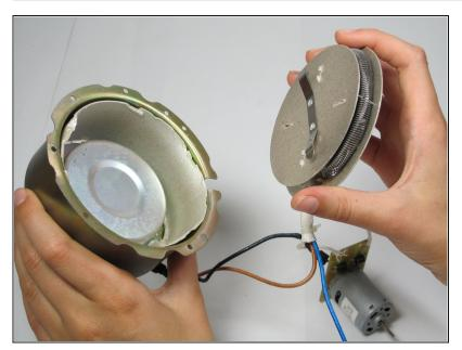
• Take the heating coil out of complete heating component.
