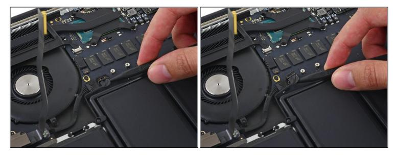
• Carefully tuck the tip of a spudger under the right speaker cable near the connector and lift it up out of its socket on the logic board.
