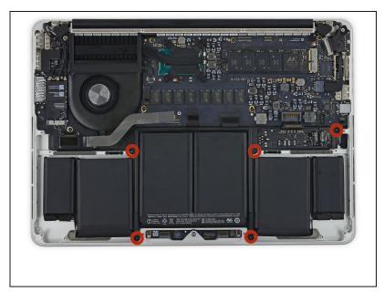
• Remove the five 3.7 mm T5 Torx screws securing the battery to the upper case.
