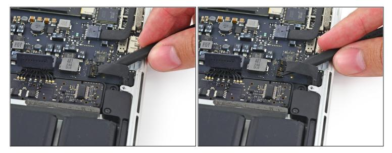
• Insert the tip of a spudger under the left speaker cable near the connector and lift it up out of its socket on the logic board.
