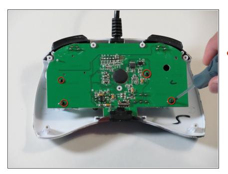
Locate the four 8.3 mm Phillips screws on the circuit board and remove them.
