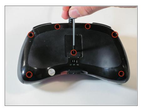
Find the seven 8.3 mm Phillips screws on the rear of the controller and remove them.
