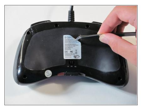
Use tweezers to completely remove the sticker from the rear of controller.
