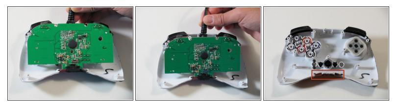
• Hold the controller cable at the area just before it meets the controller and slowly lift upwards to slide it out of its plastic slot and remove the circuit board.
