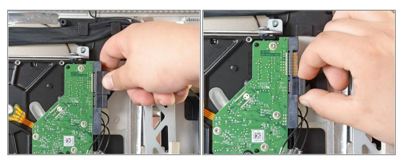
• Disconnect the SATA power and data cables from the hard drive by pulling them straight away from the hard drive.
