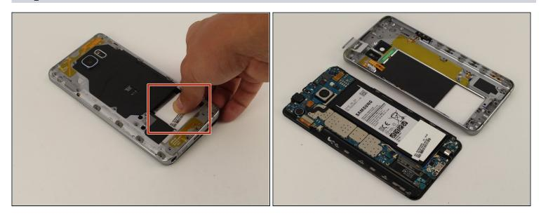
• Grip the back of the device and press down on the white square to remove the middle housing.
