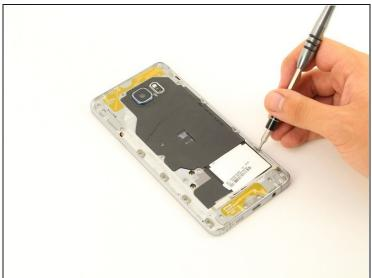
• Remove 20 5mm screws with a Phillips #1 Screwdriver.
