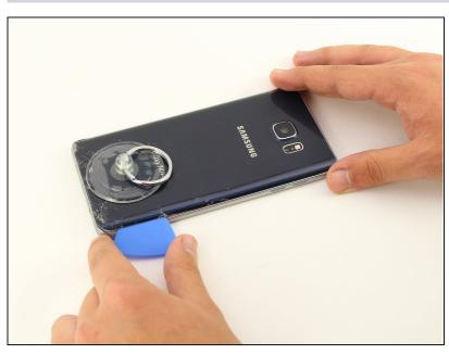
Keeping the pick under the rear glass, move the pick along the bottom edge of the device to cut the adhesive.
