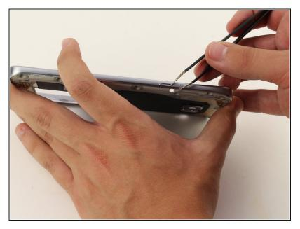
Push out the power button with the tip of the tweezers.
