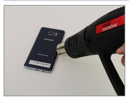
Heat the back of the device with a heat gun for 2 minutes
