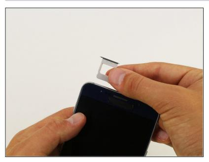
• Remove the SIM Card Tray from the slot.
