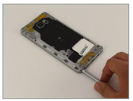
• Remove the S-Pen from the bottom of the device
