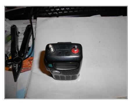
At the base of the SMA antenna connection there is a nut. Use a small straight-blade screwdriver or similar tool to loosen and unscrew the nut. Be careful not to damage the connector's threads.
