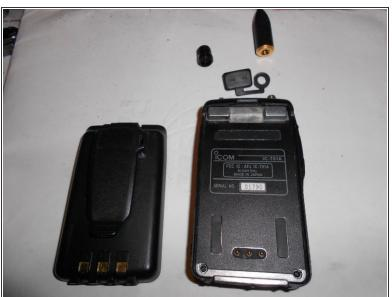
Remove the battery. Unscrew the antenna. Gently remove the rubber cover from the antenna stud.
