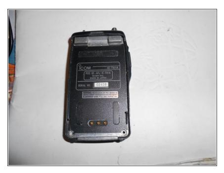
Near the bottom of the unit (under where the battery rests) there are two small Phillips screws holding the front cover to the main unit. Use the small screwdriver (and needle nose, if needed) to remove them.
