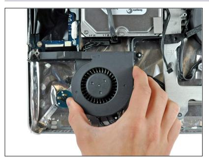
Pull the hard drive fan off the plastic posts protruding from the rear case and remove it from the iMac, minding any cables that may get caught.
