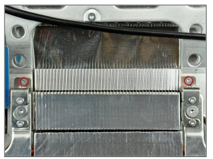
Remove the two T6 Torx screws securing the top of the heat sink framework to the chassis.
