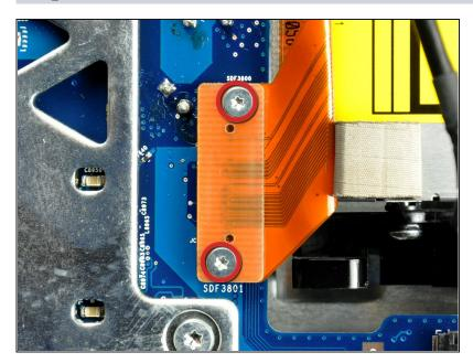
Remove the two T6 Torx screws securing the optical drive ribbon cable connector to the logic board.
