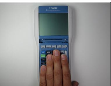
• At the same time, slide the latch to the right and pull the keypad downward. This should completely separate the keypad from the calculator.
