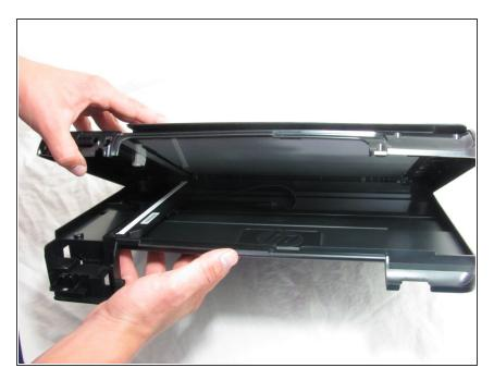
• Pull the printer hood upward.
