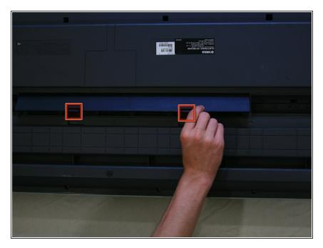
Pop the tabs on the battery casing and remove it from the back plate.
