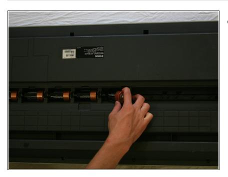
Locate the six batteries and remove them from the battery cavity.
