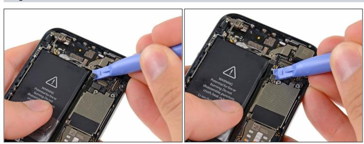
• Use a plastic opening tool to pry the two interconnect cables up from their sockets at the top of the logic board.
