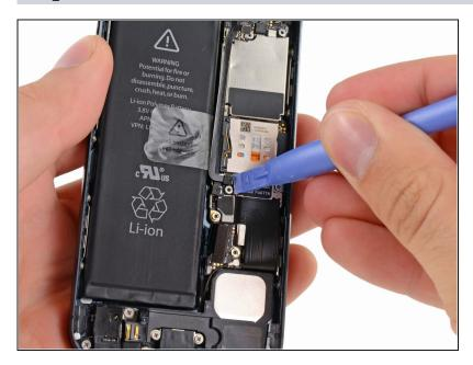
Disconnect the two interconnect cables from the bottom of the logic board in the same manner described above.
