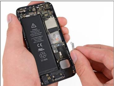
• Remove the metal bracket securing the battery connector from the iPhone.
