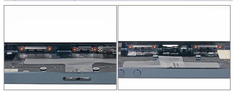
• The four front panel clips are held in with two 1.3 mm Phillips screws each. Remove the screws on the clip(s) you want to replace.
