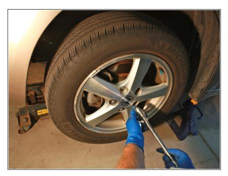
Once car is raised, remove the lug nuts on one of the front tires with the 3/4" socket.
