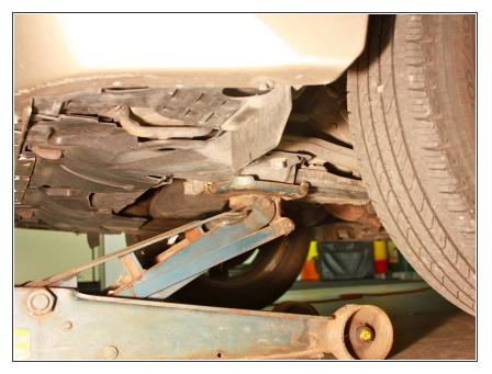
Push downward on the jack's lever to lift the saddle upward so that it contacts the crossmember. Continue pushing downward on the lever to lift the car upward.
