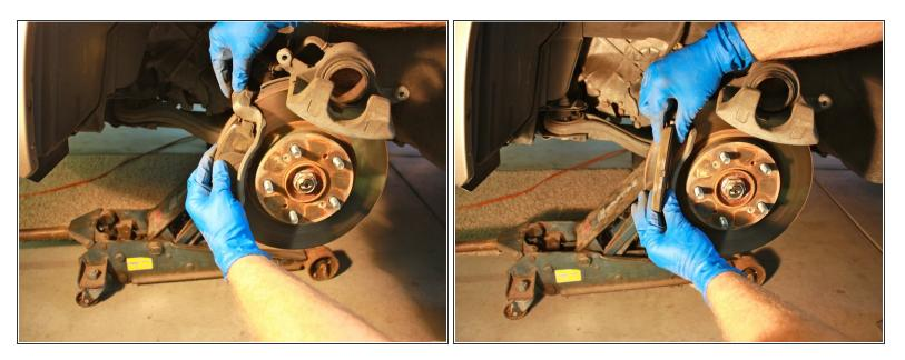
• Pull the two old brake pads out of both the front and rear of the pad bracket.
