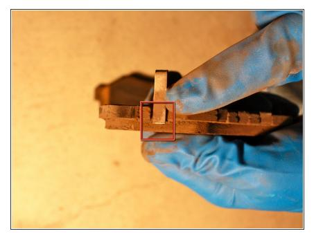
Inspect the brake pad wear sensor on the old brake pad. The sensor is a metallic tab attached to the brake pad. When the brake pads wear down too much, the metallic tab contacts the rotor and makes a screeching sound.
