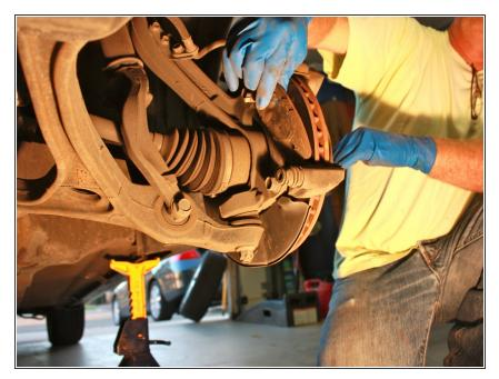
Place the new brake pads into the bracket. Make sure that the new pads are secure.
