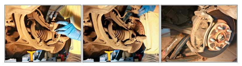
• Slide the caliper off and rest it on the top of the rotor.
