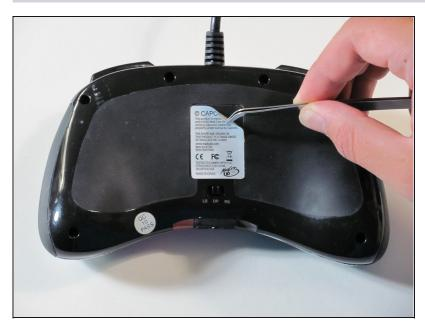
• Use <u>tweezers</u> to completely remove the sticker from the rear of controller.
