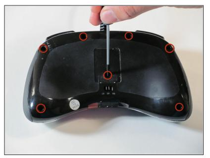
• Find the seven 8.3 mm Phillips screws on the rear of the controller and remove them.
