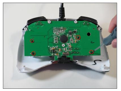
Locate the four 8.3 mm Phillips screws on the circuit board and remove them.
