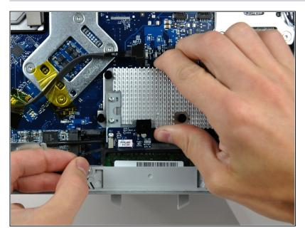
• De-route the speaker cables from beneath the IR Board and heatsink assembly.
