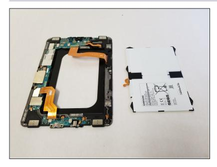
• The battery should now be removed and detached from the device.
