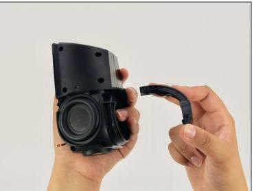
• Using a Torx T6 screwdriver head, unscrew the six black 1.7mm Torx screws on the side of the device.
