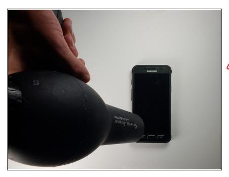
Melt the adhesive on the screen by applying a blow dryer directly on the screen.
