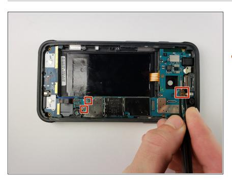
Use tweezers to disconnect the front mic and the two cables that have been marked in the photo.
