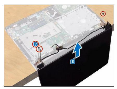
Remove the three screws (M2.5x8) that secure the display-hinge brackets to the palm-rest assembly.
