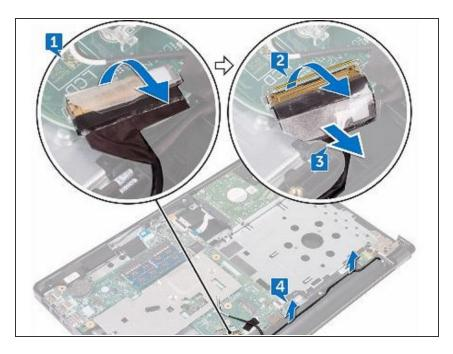
• Close the latch that secures the display cable to the system board.
