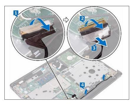
• Adhere the tape that secures the display cable to the system board.
