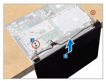
• Replace the three screws (M2.5x8) that secure the display hinges to the palm-rest assembly.
