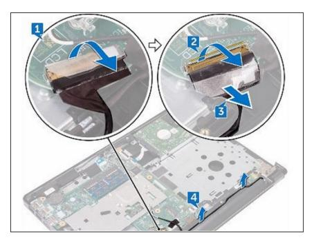
Note the antenna-cable routing, and remove the antenna cable from the routing guides on the palm-rest assembly.
