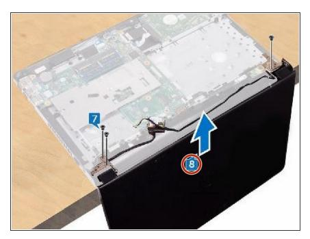
• Carefully place the display assembly on a clean and flat surface.
