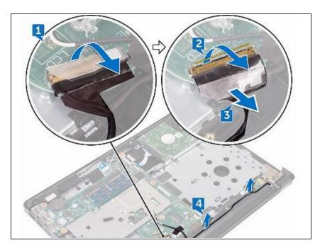
• Connect the display cable from the system board.
