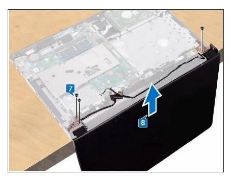
• Place the **NEW** display assembly at the edge of the table.
