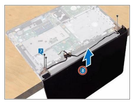
• Carefully lift the display assembly from the palm-rest assembly.
