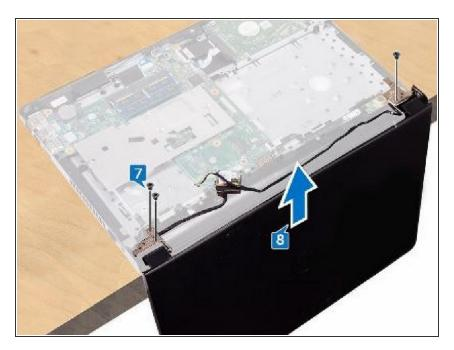
Align the screw holes on the palmrest assembly with the screw holes on the display hinges.
